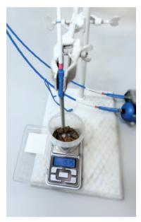
Narrow spectral bands are used to obtain information on the humus content. As a source of radiation and sensitive elements, photo- and light-emitting diodes are used.
